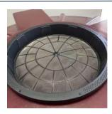
The use of a light guard or cover can be used to reduce the effect of algae growth.
